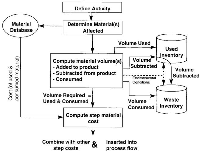
Fig. 1. Modeling process for treating material addition and subtraction. The environmental conditions are necessary to convert the material volumes to STP. The material database provides material cost and waste disposition information.
