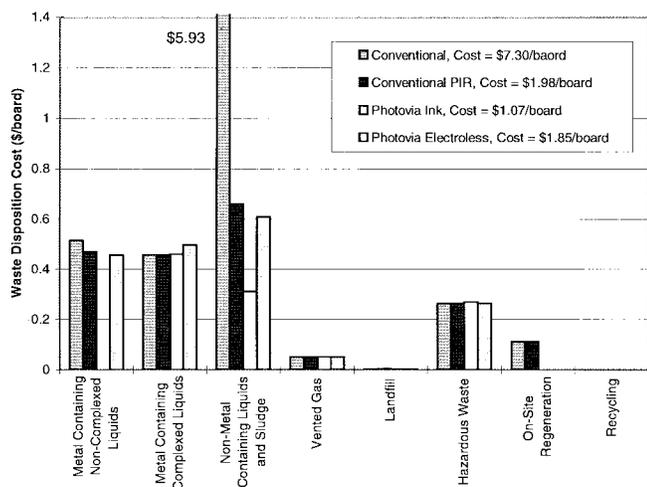
Fig. 15. Waste disposition cost versus activity comparison of 8 layer conventional board and 6 layer photovia board fabrication processes.
