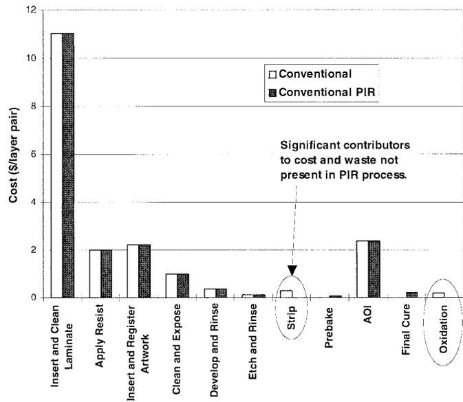
Fig. 8. Cost of conventional and PIR layer-pair fabrication including oxide treatment, excluding waste disposition. (The actual process models used consist of ~30 process steps that have been combined in this figure for convenience.)
