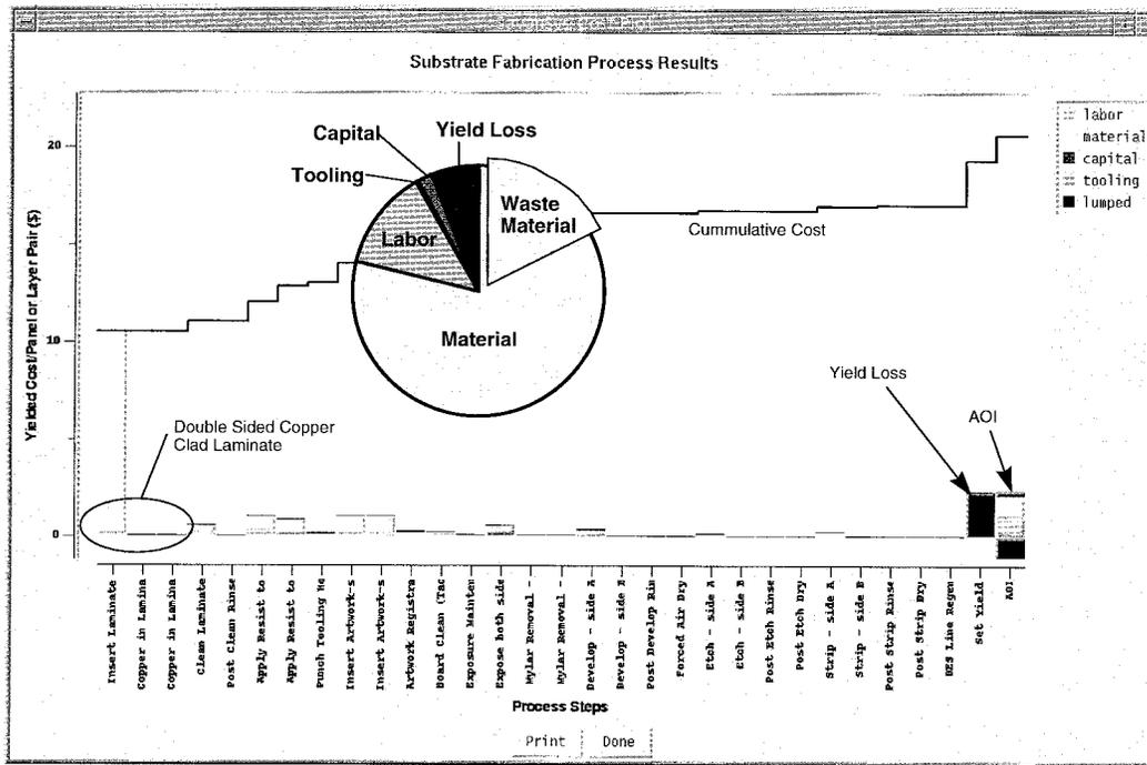
Fig. 5. Cost as a function of process step for the fabrication of a double-sided, undrilled, copper clad layer-pair. The embedded pie chart shows the fractional distribution of labor, material, tooling, and capital costs. The portion of the material cost that ends up being wasted is shown as a raised pie slice.
