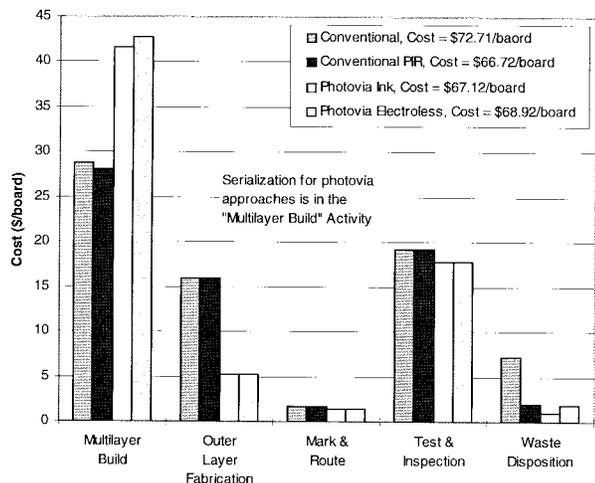
Fig. 14. Cost versus activity comparison of eight layer conventional board and six layer photovia board fabrication processes.
