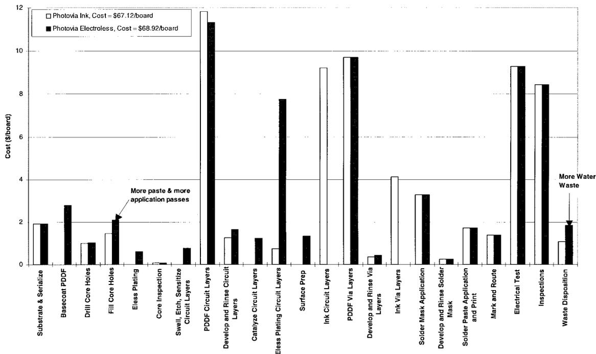
Fig. 12. Cost of ink and electroless metallization fully-additive photovia PWB fabrication processes including waste disposition. (The actual process models used consist of 250–350 process steps that have been combined in this figure of convenience.)
