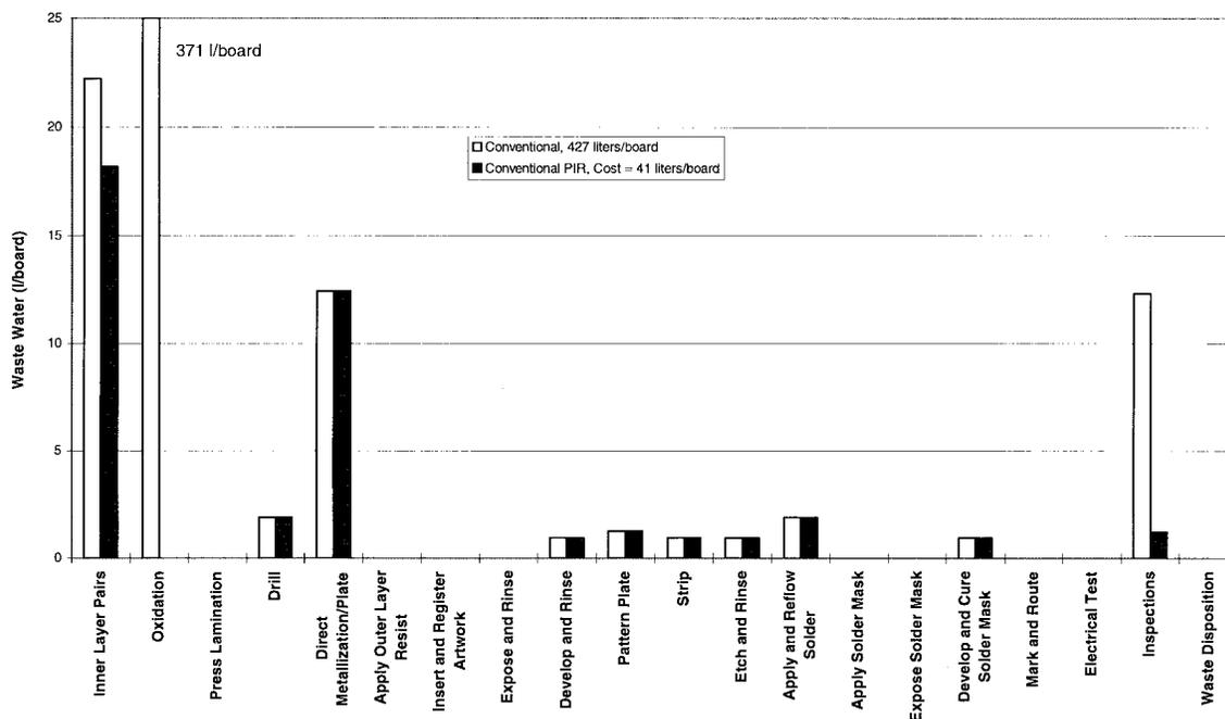
Fig. 11. Waste water of conventional and PIR full multilayer build. (The actual process models used consist of  $\sim 230$  process steps that have been combined in this figure of convenience.)
