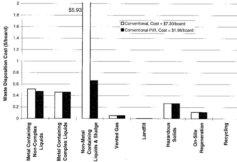
Fig. 10. Waste disposition costs as a function of material category. The “nonmetal containing liquids and sludge” category includes water.
