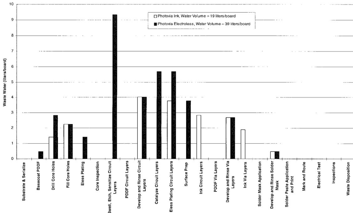
Fig. 13. Waste water of ink and electroless metallization fully-additive photovia PWB fabrication processes including waste disposition. (The actual process models used consist of 250–350 process steps that have been combined in this figure of convenience.)
