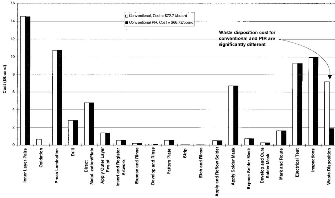
Fig. 9. Cost of conventional and PIR full multilayer build including waste disposition. (The actual process models used consist of ~230 process steps that have been combined in this figure of convenience.)
