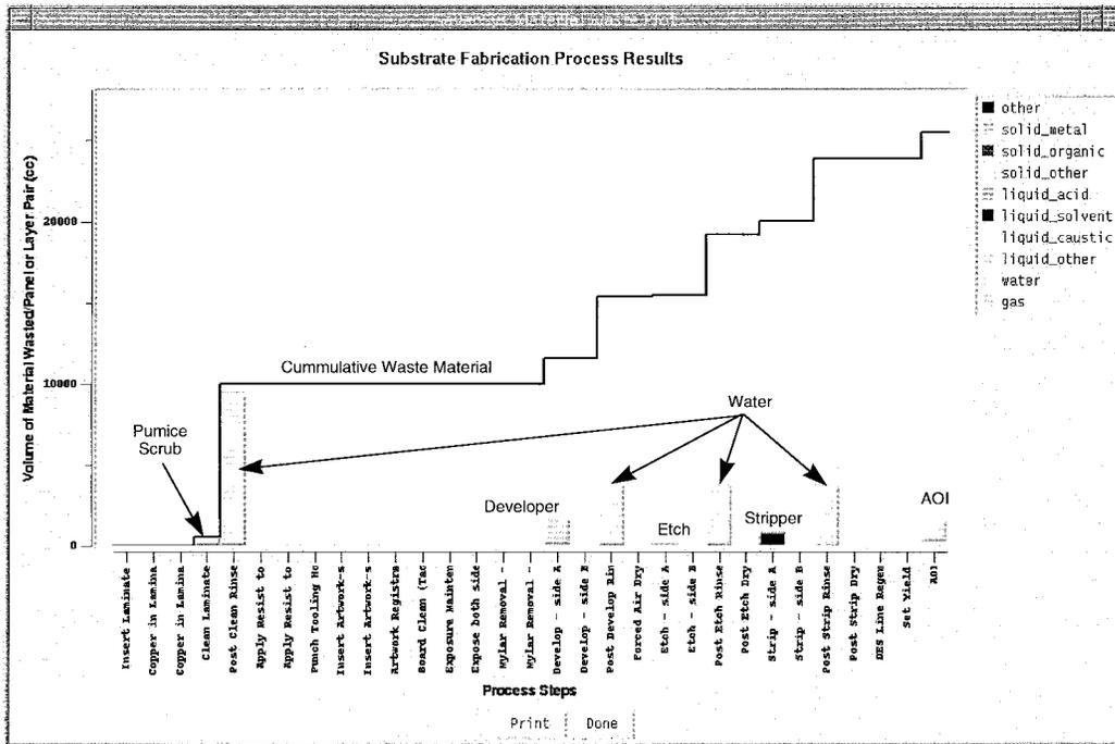
Fig. 7. Material wasted as a function of the process steps associated with fabricating a double-sided, undrilled, copper clad layer-pair.
