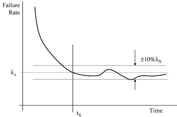
Fig. 3. Change point estimation for  $t_s$ ,  $\lambda_s$  is the failure rate at  $t_s$ .
