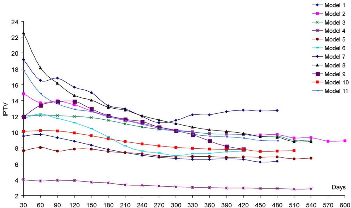
Fig. 2. Failure rates expressed in incidents per thousand vehicles (IPTV) for selected passenger compartment mounted electronic products recorded by Delphi Corporation. The actual IPTV values have been modified to protect the proprietary nature of the data.
