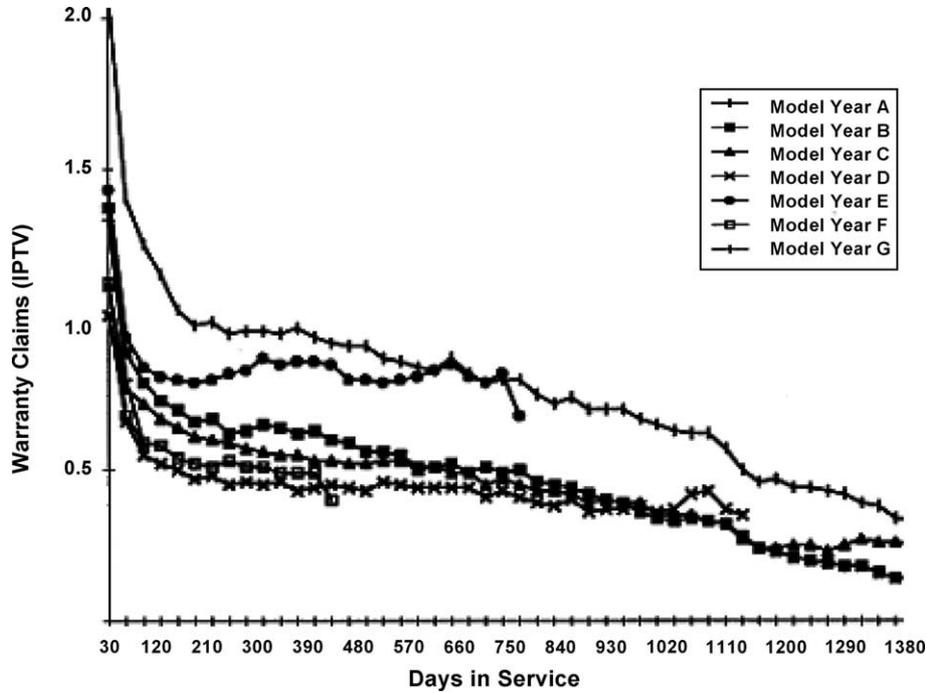
Fig. 1. Extended warranty charts compiled from Delphi Corporation warranty data for the several model years of the same electronic product mounted in the engine compartment of an automobile.
