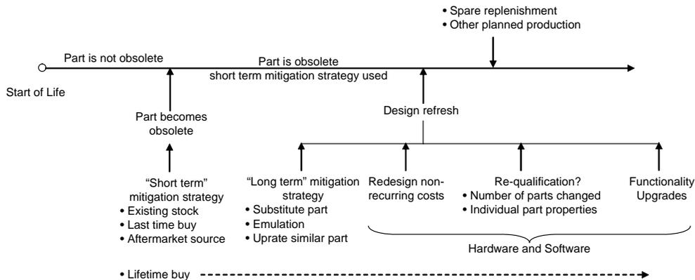
Fig. 5. Design refresh planning analysis timeline (presented for one part only, for simplicity, however in reality, there are coupled parallel timelines for many parts, and design refreshes and production events can occur multiple times and in any order), [5].
