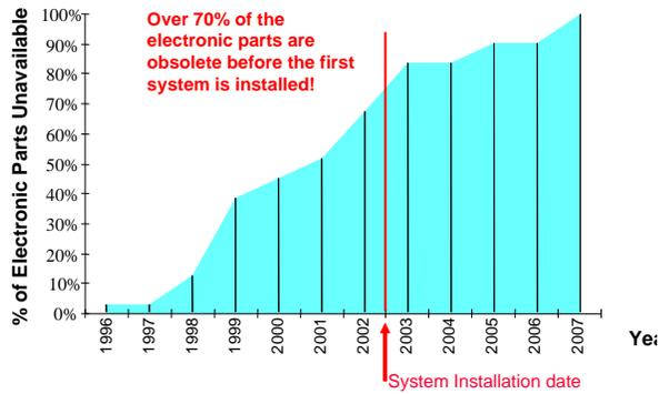
Fig. 1. Portion of the Commercial Off The Shelf (COTS) electronic parts that become un-procurable in the first 10 years of a surface ship sonar system's life cycle (Courtesy of NAVSURFWARCENDIV Crane, [5]).
