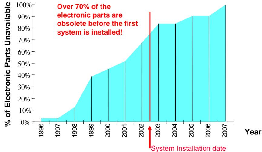
Figure 2: Percent of Commercial Off The Shelf (COTS) parts that are out of production (un-procurable) versus the first 10 years of a surface ship sonar system's life cycle (courtesy of NAVSURFWARCENDIV Crane)
