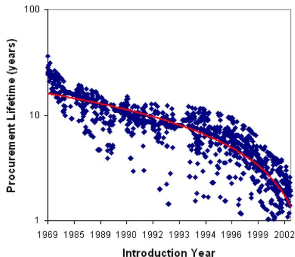
Figure 1: Decreasing procurement lifetime for operational amplifiers, an electronic part common to nearly every electronics application, [2] (the procurement life is the number of years the part can be procured from its original manufacturer)
