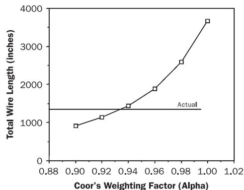
Figure 5 shows the results using the statistical wire length distribution method where the calibration factor is the value of  $\alpha$ . The method overestimates the wiring length needed by 8.3 percent when using the 50mil pad placement grid size used in the actual routing.
