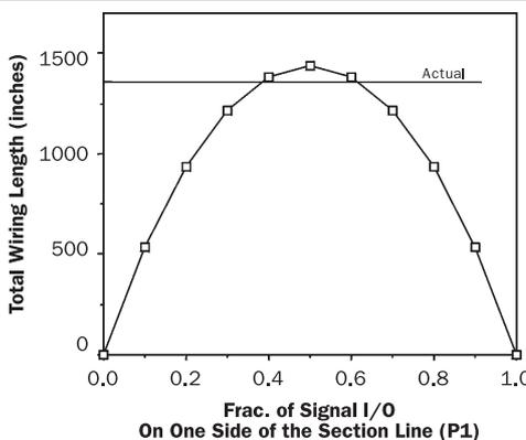
The calibration factor in the section-crossing model is the fraction of I/O on one side of the section line ( $P_1$  or  $P_2$ ). In this comparison approach we have only computed the length of a single cross-section of the board (assumed that the area of the board is the length of that section squared). The section-crossing method shown in Figure 4 returns reasonable results for this example case ( $P_1 = 0.5$ , overestimates the total wire length by 8.6 percent).
