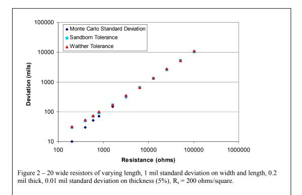
As can be seen in Figure 2, the tolerance calculations match the actual standard deviation prediction for large resistors and over-predict the standard deviation for smaller resistors. The relation shown in Figure 2 is a function of the standard deviations on the width, length, and thickness. For example, the same data with a thickness standard deviation of 0.03 mils is shown in Figure 3.
