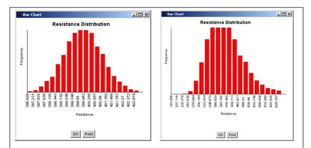
Figure 1 – 20 mil x 40 mil resistor, 1 mil standard deviation on width and length, 0.2 mil thick,  $R_s = 200$  ohms/square. Left 0.01 mil standard deviation on thickness (5%), right 0.03 mil standard deviation on thickness (15%).
