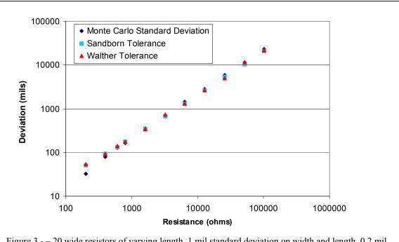
Figure 3 - -20 wide resistors of varying length, 1 mil standard deviation on width and length, 0.2 mil thick, 0.03 mil standard deviation on thickness (15%),  $R_s = 200$  ohms/square.
