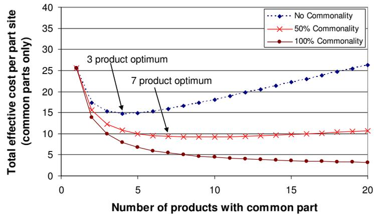
Figure 11. 1 to 20 products concurrently using the example part described in Figure 2. Problem introduced in year 5, total quantity of each product = 12,910.
