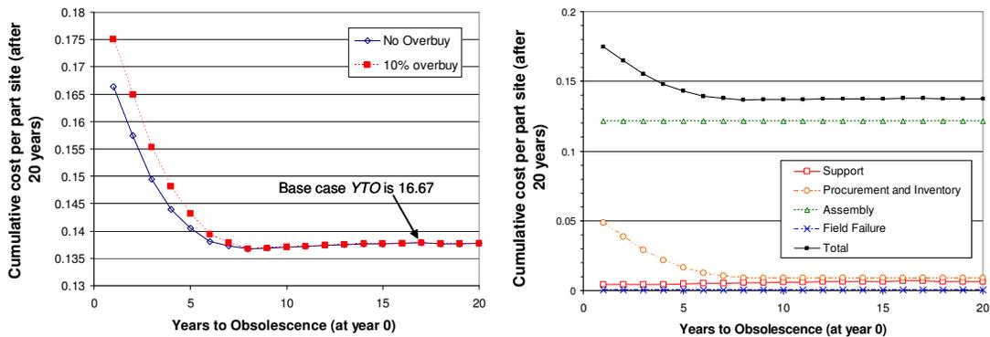
Figure 6. Cumulative cost per part site as a function of part procurement life ( $YTO$ ) for (left) 0% and 10% overbuy on lifetime buys, and (right) 10% overbuy with respect to cost category.
