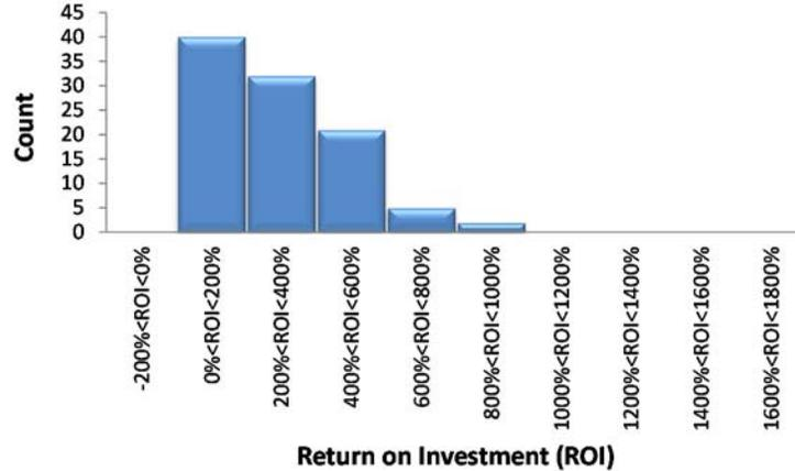
Fig. 15. Histogram of ROIs for the commercial aircraft,  $\eta = 50,000$  cycles, activities performed at the highest level of rigor (level 5).
