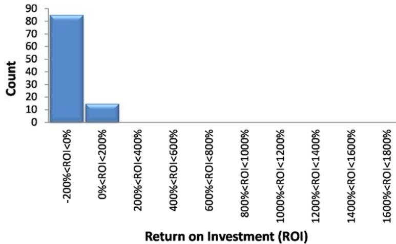
**Fig. 17.** Histogram of ROIs for the commercial aircraft,  $\eta = 50,000$  cycles, activities performed at level of rigor 3, activities are not independent.
