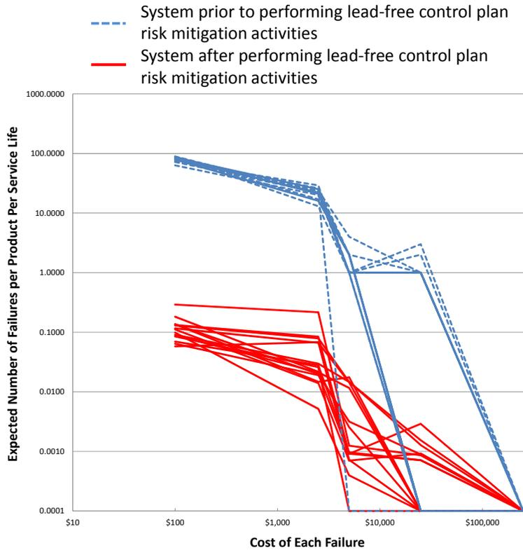
Fig. 14. Results for commercial aircraft,  $\eta = 50,000$  cycles, activities performed at the highest level of rigor (level 5).
