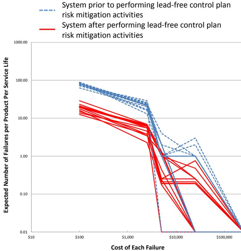
Fig. 18. Results for the commercial aircraft,  $\eta = 50,000$  cycles, activities performed at level 5 of rigor, activities are not independent.
