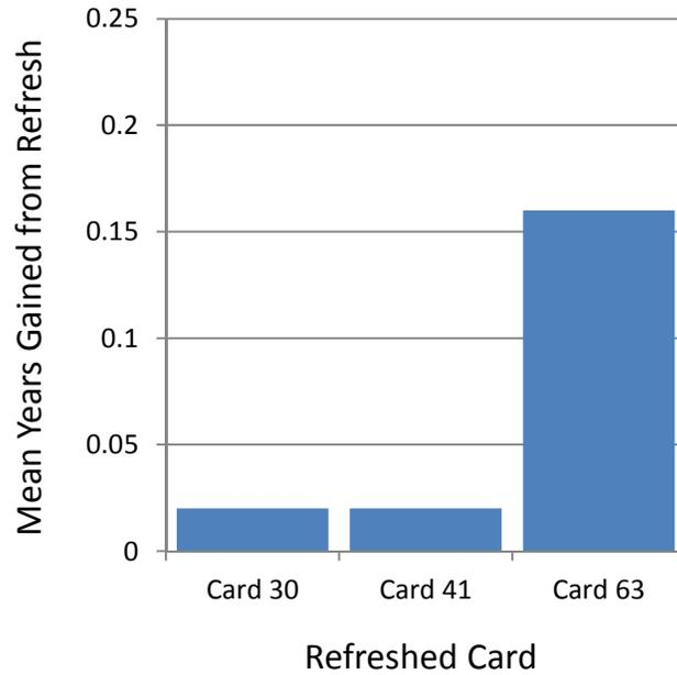
**Fig. 13 System support life gained from individual card refresh, case 2.**
