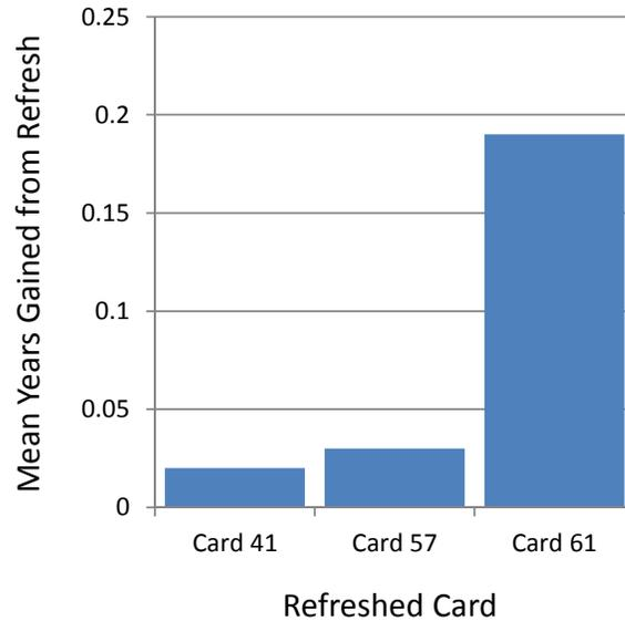
**Fig. 14 System support life gained from individual card refresh, case 3.**
