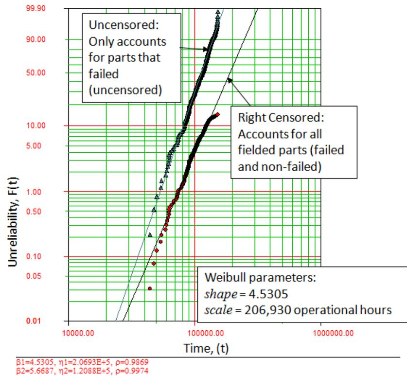
**Fig. 5 Part number 5004-02 failure distribution. Both data sets are equal, one shows 10% unreliable, the other 100% unreliable (censored versus uncensored).**
