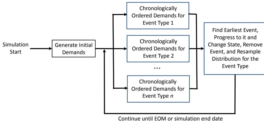
**Fig. 2 Discrete-event simulation flow for multiple events.**
