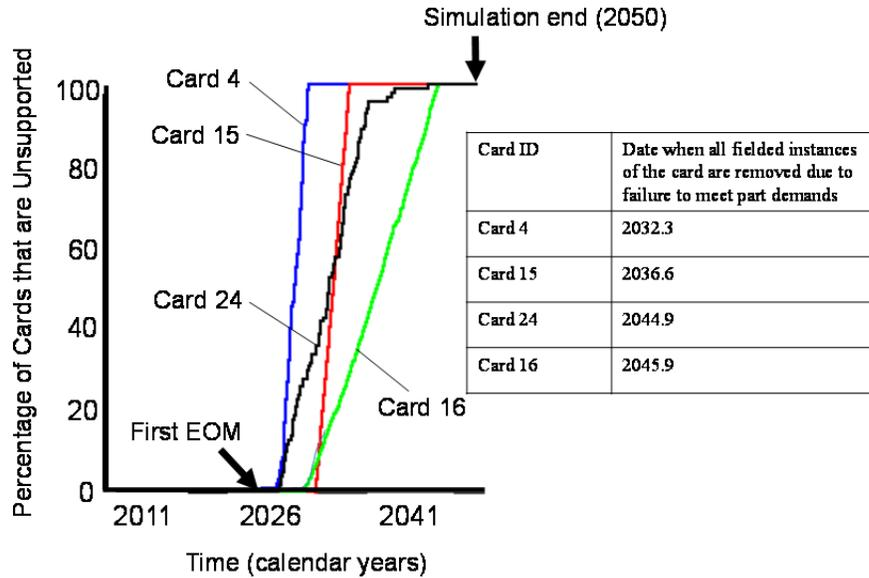
**Fig. 9 Card-level support tracking and loss.**
