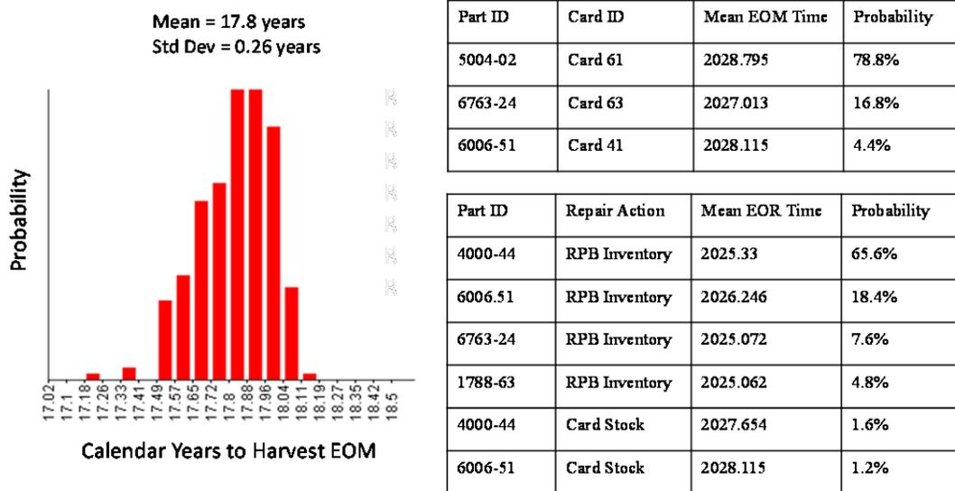
Fig. 8 System-level EOM distribution (left), EOM (top right) and EOR (bottom right) results for Case 3.
