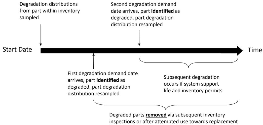
**Fig. 3 Part degradation in inventory (shelf-life) process flow for a single part.**
