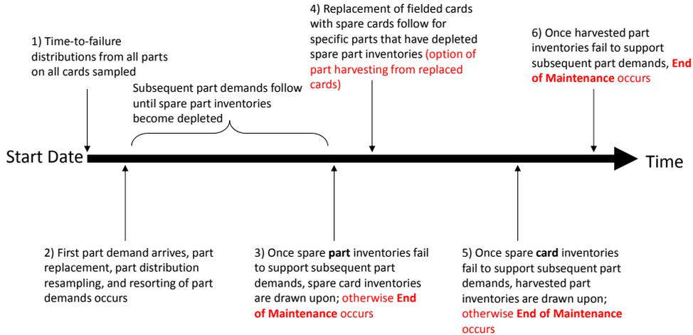
**Fig. 1 EOR/EOM part failure process flow (single life history).**
