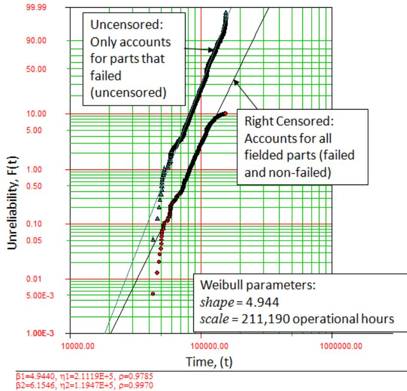
**Fig. 4 Part number 3798-05 failure distribution. Both data sets are equal, one shows 10% unreliable, the other 100% unreliable (censored versus uncensored).**
