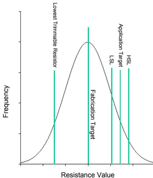
Figure 2 – Distribution of fabricated resistor values.
