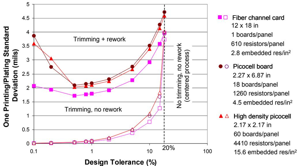
Figure 3 – Application-specific economical regions of trimming and reworking embedded resistors. This example result assumes no resistor thickness variation, see [13] for additional assumptions and modeling parameters associated with this result.
