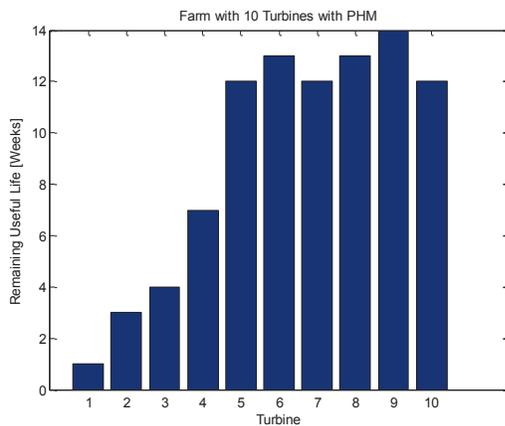
Figure 2- Turbines with different prognostic indication
