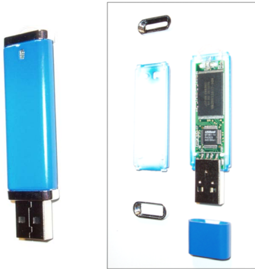
Fig. 5. 128MB USB flash memory drive prior to disassembly – left, disassembled – right. The overall dimensions are approximately 2.5 x 0.75 x 0.375 inches.
