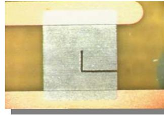
**Figure 2** Trimmed Metal Thin film
