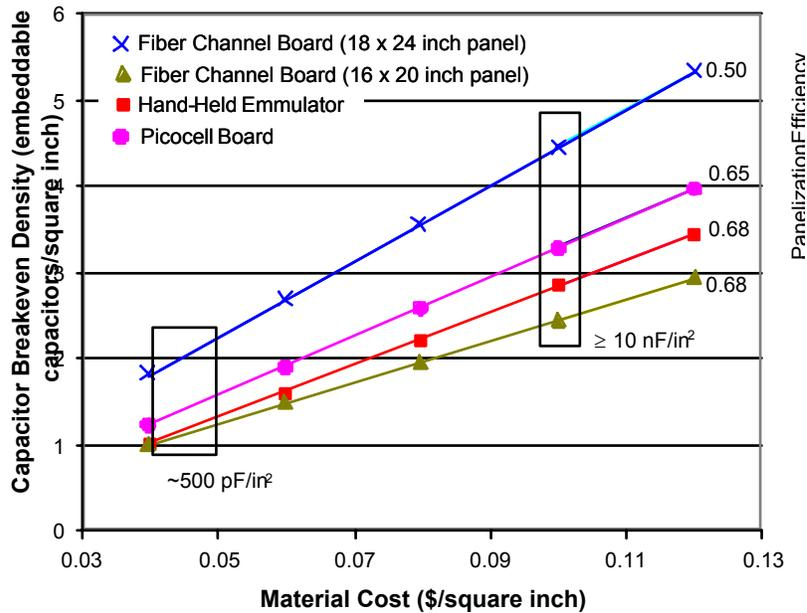
Figure 6 - Bypass capacitor breakeven densities in capacitors/in<sup>2</sup> as a function of dielectric material capacitance and replacement costs, and panel use efficiency.
