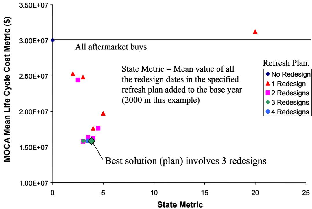
**Figure 7.** MOCA design refresh solution for the AS900 FADEC. This solution assumes: 1 year look-ahead time, 200 component re-qualification trigger, and \$136,000 full re-qualification cost.
