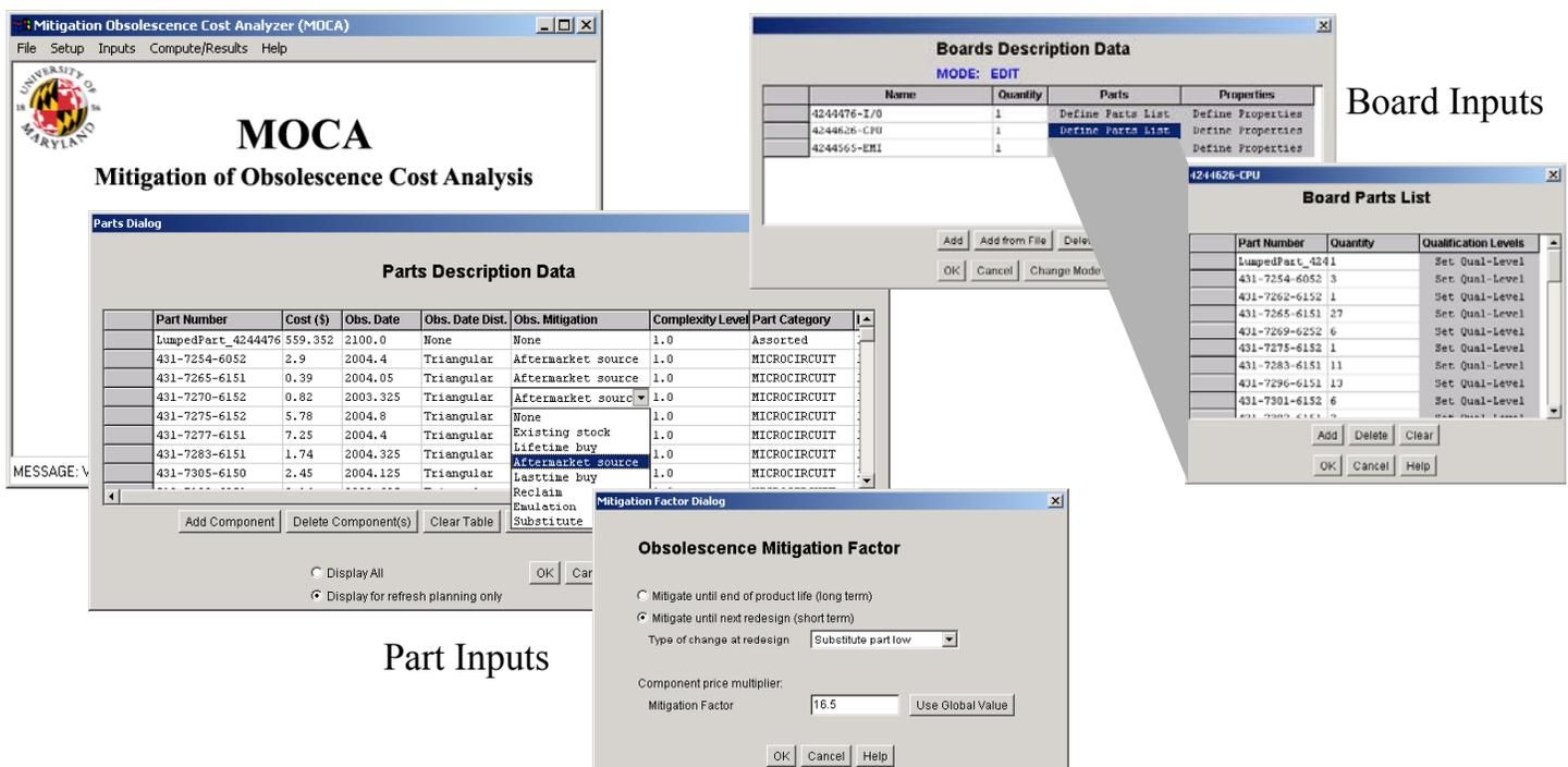
Figure 2. MOCA part and board-level input interfaces.
