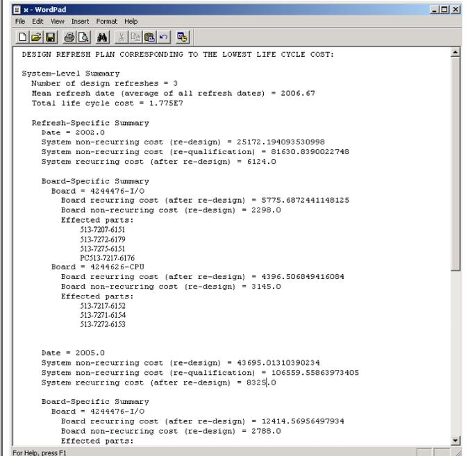
**Figure 5.** Example output from the MOCA tool. Left = results plot with one refresh plan expanded, right = the actual refresh plan corresponding to the expanded point.
