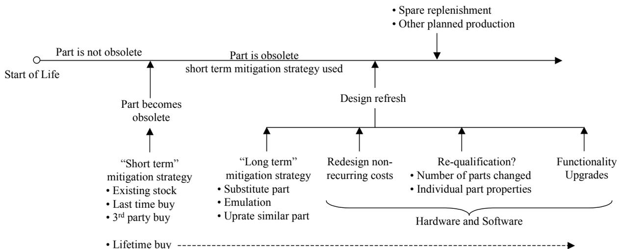
**Figure 1.** Design refresh planning analysis timeline (presented for one part only, for simplicity, however in reality, there are coupled parallel timelines for all the parts in the product).
